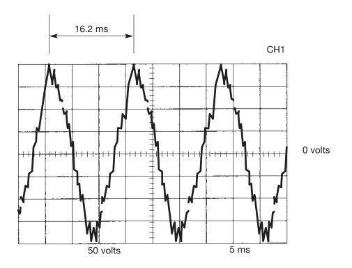
This is the typical AC output voltage generated from a properly operating machine. Note that each vertical division represents 50 volts and that each horizontal division represents 5 milliseconds in time.
